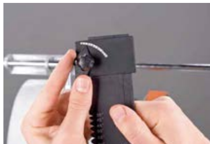
2. 设置裁切实际角度 Step 2: Setting the measured angle of cut.
