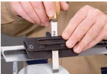
0-30°角度的研磨 Grinding at angles between 0-30°
