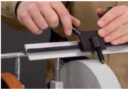
修整砂轮 Dressing the grinding stone
