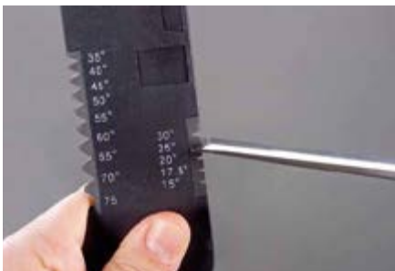
1. 检查并判定裁切角 Step 1: Check and determine the cutting angle.
