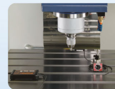
■ Ball bar inspection
