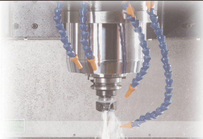
■ Belt type / Direct-drive spindle, 11/15kW, 12000rpm (Optional)
