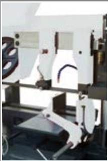
锯条支承调整 Saw blade holder adjustment
