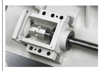
To eliminate lost motion, the ballscrews are double nut type, anchored on both ends and pretensioned. The motors are directly coupled to the ballscrews.
