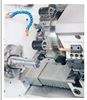
The 10 station slotted disk turret takes conventional "stick" tooling with wedge clamps
