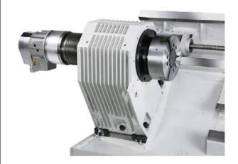
The headstock is of rugged construction to enable heavy cutting with maximum stability. The ribbed design provides excellent heat dissipation and helps reduce thermal deformation of the spindle
