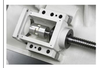
To eliminate lost motion, the ballscrews are double nut type, anchored on both ends and pretensioned. The motors are directly coupled to the ballscrews.
