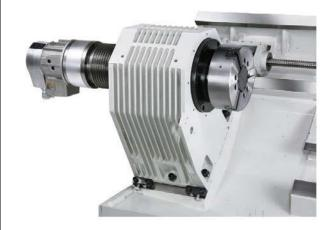
The headstock is of rugged construction to enable heavy cutting with maximum stability. The ribbed design provides excellent heat dissipation and helps reduce thermal deformation of the spindle
