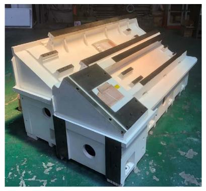
The solid one-piece Meehanite casting with strategic rib reinforcement dampens vibration, and increases structural strength.
