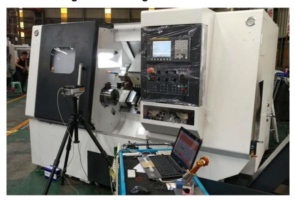
After assembly, Takumi lathes are thoroughly tested – including the use of a laser interferometer. This provides comprehensive accuracy assessment of machine alignment and any roll-pitch-yaw errors in machine
