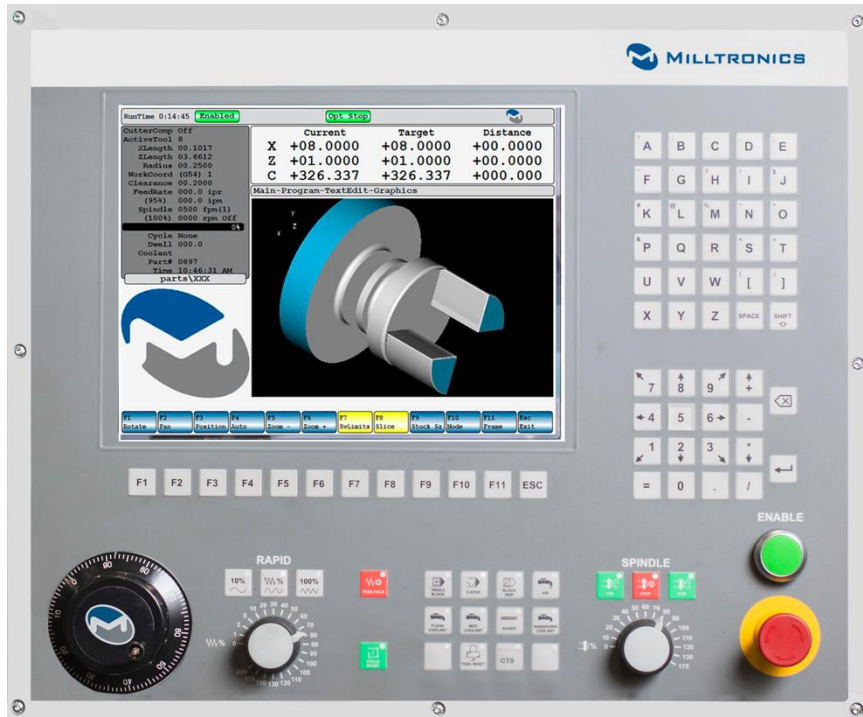
Series 8220-B control is Linux-based and features a 12" color LCD screen
